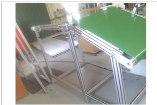
CE-OP001-Inclined Conveyor Belt
